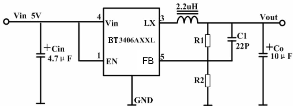
$$V_{out} = 0.6 * (1 + \frac{R_1}{R_2})$$
