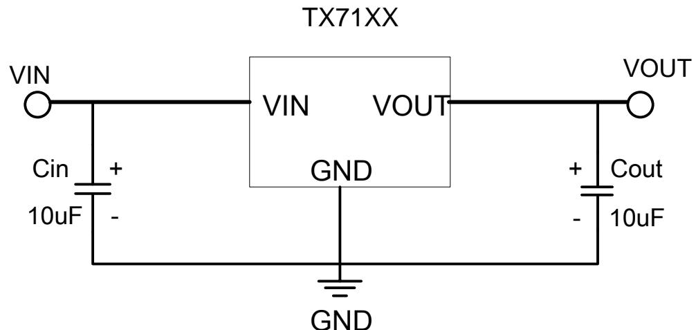
Note1:  $C_{in}=C_{out}=10\mu F$ . (10uF Electrolytic capacitor is recommended).
